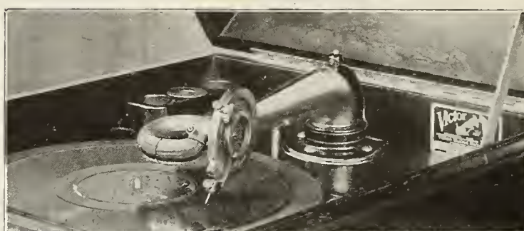
Showing Blood Reproducer in position for playing Lateral Cut records on the Victor Phonograph. Large diaphragm insures natural, lifelike reproduction.
